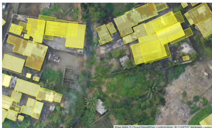
Figure 2: Missed labelling on buildings near trees (Pointe-Noire, Congo)
